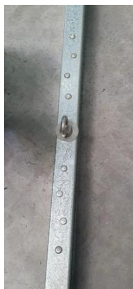
Step-8: Use rivet tool to install all the rivets.
