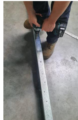
Step-3: Use 8mm drill bit to drill holes at 8 rivets locations.
