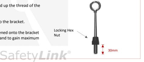
**EYEBOLTS** - Threads need to have a minimum of **SIX FULL 360**° **TURNS** into the ultimate thread. **RETRO EYEBOLTS** - Threads need to have a minimum of **EIGHT FULL 360**° **TURNS** into the ultimate thread.
