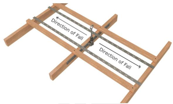
Bracing may be required for sideways loads due to rafter size, location of rafter (high in the hip) and existing additional structural bracing (existing batten locations, noggins, metal bracing, plywood decking). Assessment will always need to be made by a competent person for each anchor installation at time of install.
