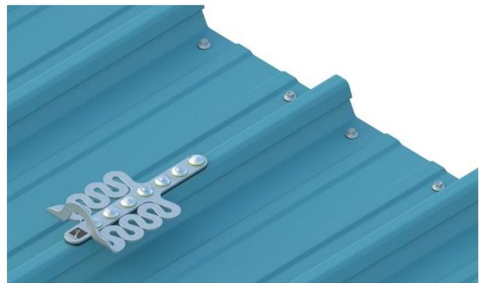
**FROGLINK INSTALLED LESS THAN 2M FROM ROOF SHEET EDGES REQUIRE 4X12G ADDITIONAL SCREWS TO SECURE ROOF SHEETS INTO PURLIN ON SIDE THAT FALLS UNDER 2M**
