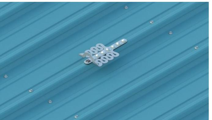
**FROGLINK INSTALLED LESS THAN 2M FROM BOTH SIDES OF ROOF SHEET EDGES REQUIRE 4X12G ADDITIONAL SCREWS TO SECURE ROOF SHEETS INTO PURLINS ON BOTH SIDES THAT FALL UNDER 2M**
