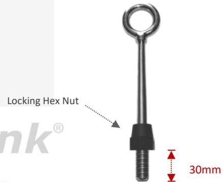
**EYEBOLTS** - Threads need to have a minimum of **SIX FULL 360° TURNS** into the ultimate thread.
