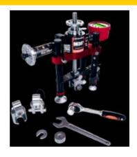
The upgraded Hydrajaws Safety Lifeline Cable Tester KIT 2 is a complete kit enabling engineers to validate the installation of anchors, eyebolts up to a maximum tensile load of 35kN and swaged components on newly installed or existing engineered lifeline systems to ensure compliance with BS 7883, up to a maximum tensile load of 20kN.
